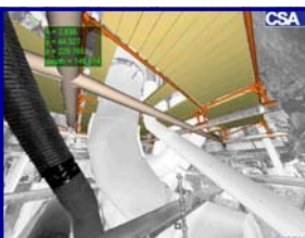
Above, 3D Modeling of the Scaffold Design, performed by CSA Laser Associates.
