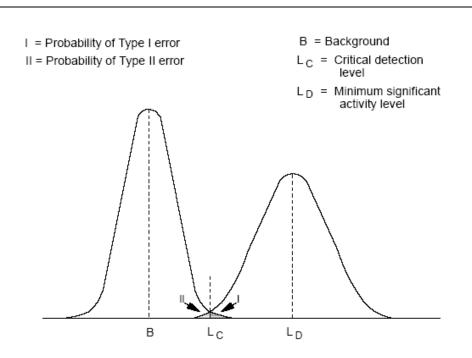
Figure 6. Errors in Detection Sensitivity
