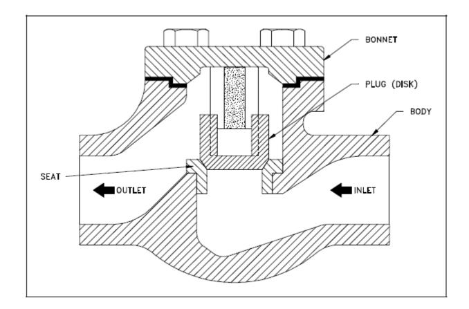
Lift check valves are suitable for installation in horizontal or vertical lines with upward flow. They are recommended for use with steam, air, gas, water, and on vapor lines with high flow velocities. These valves are available in three body patterns: horizontal, angle, and vertical.
