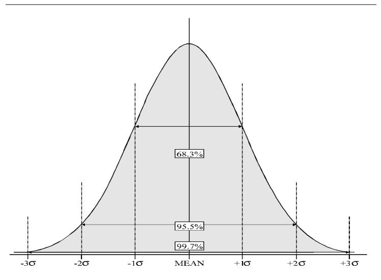
NOTE: The Normal or Gaussian Distribution Curve percentages indicate that 68.3% of the observations will be in error by less than + 1 sigma, 95.5% of the observations will be in error by less than + 2 sigma, and 99.7% of the observations will be in error by less than + 3 sigma.
